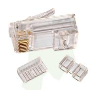
link lengths exceed 10 Meters, a horizontal cable type is specified. Horizontal cable is normally made with solid conductor copper wire in the diameter range of AWG 23 through AWG 24. This larger copper size translates into larger conductor diameters which make terminating to a traditional modular plug problematic. EngineerPro® cat6A Modular Plug design accommodates this large diameter cabling in the form factor of a standard RJ45 plug.
